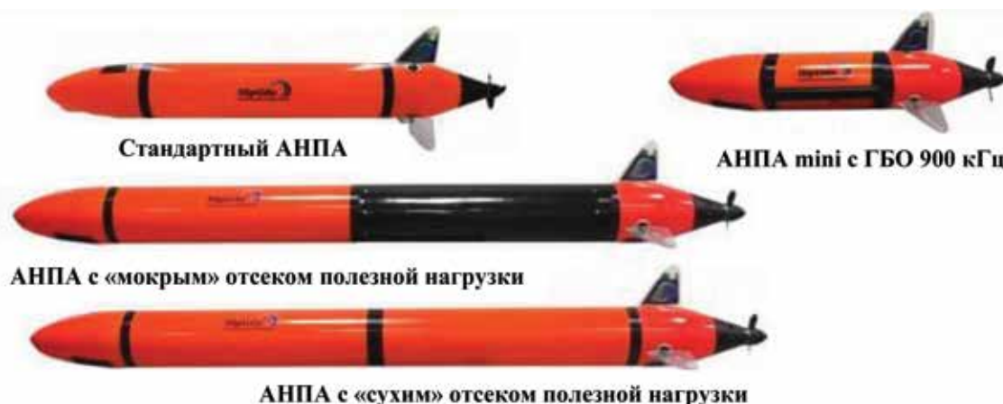
Рис. 1. Micro-UUV фирмы Riptide Autonomous Solutions
